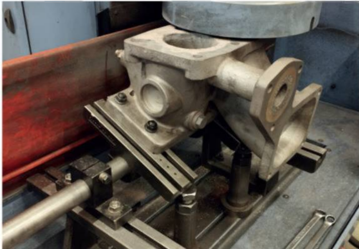
MEDIUM SPEED ENGINE – INJECTOR SLEEVES' BORE MACHINING
