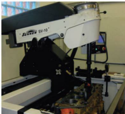
HIGH SPEED ENGINES - HONING OF THE CYLINDER LINERS
