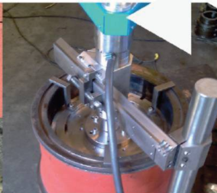
CYLINDER LINER'S LANDING SURFACE GRINDING
