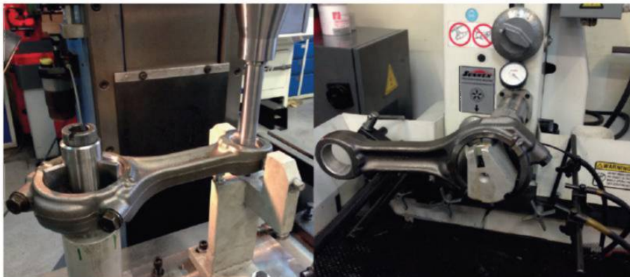
HIGH SPEED ENGINES - MACHINING OF THE CONNECTING ROD'S SMALL END BEARING
