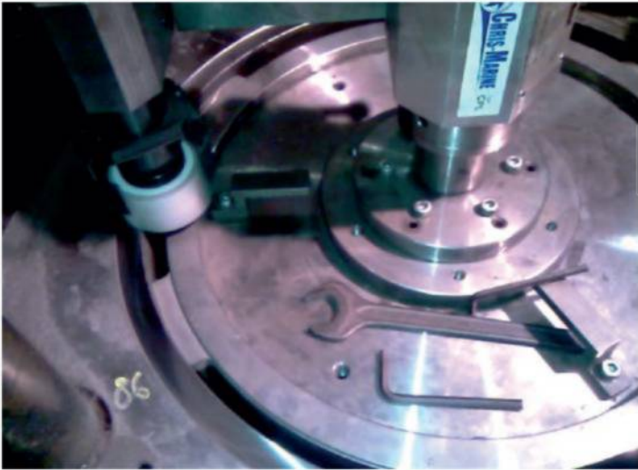
HIGH SPEED ENGINE - CYLINDER HEAD VALVE SEATS MACHINING
