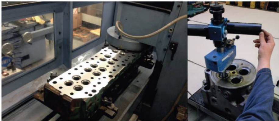
CYLINDER HEAD'S LANDING SURFACE MACHINING
