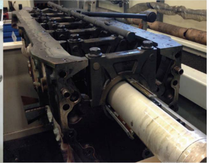
CYLINDER BLOCK - HONING OF THE MAIN BEARING CAPS
