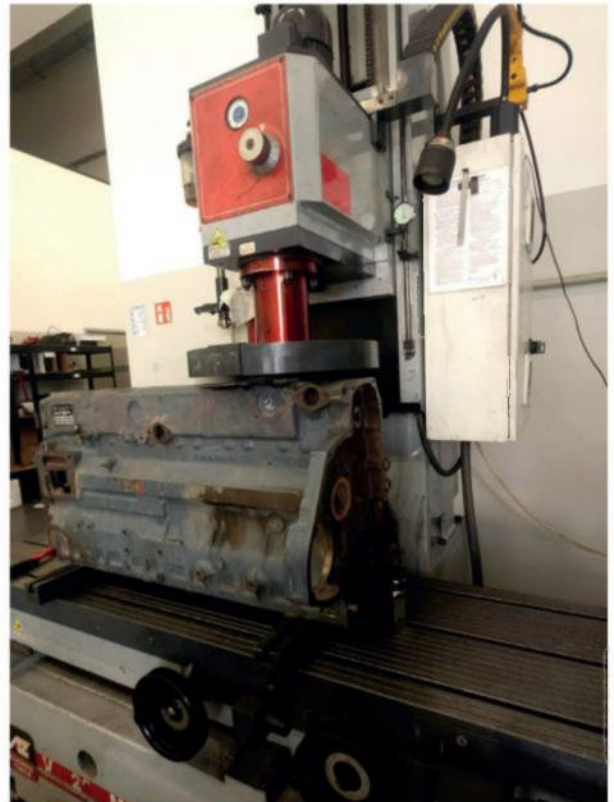
CYLINDER BLOCK'S TOP DECK MACHINING
