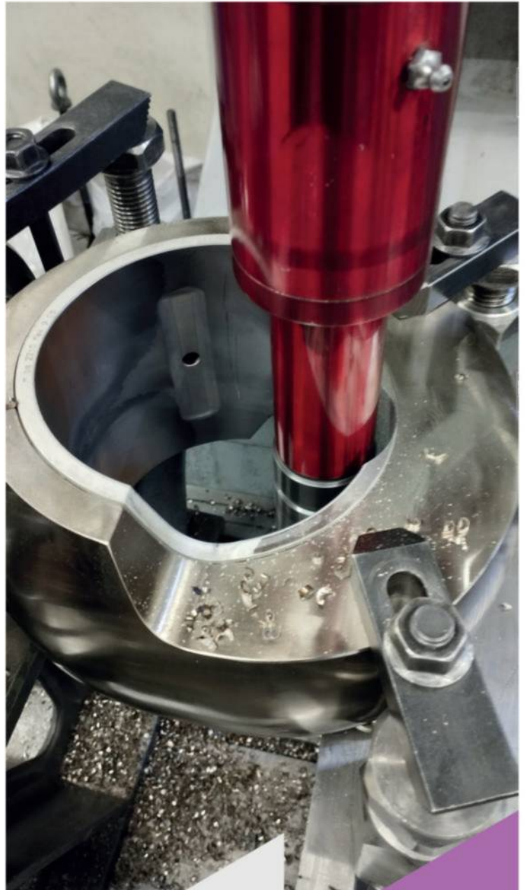
SMALL END BEARING BUSH REPLACEMENT BY MILLING
