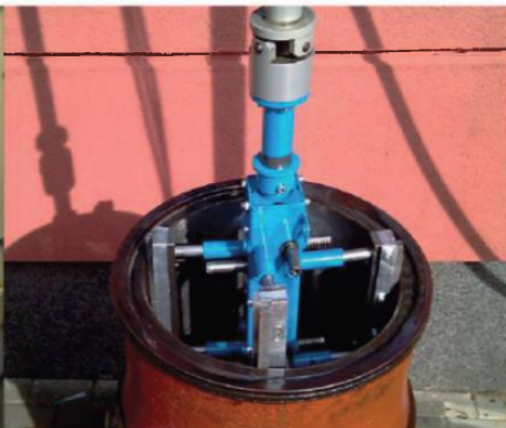
HONING OF THE CYLINDER LINER
